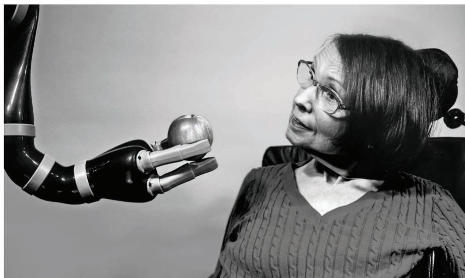
A paralyzed individual uses a brain-computer interface to manipulate an apple with a robotic arm.
